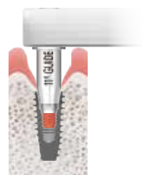
Place Guide at Fixture Connection ※ Make sure connection is secure
