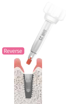
Pick up with Screw Holder and remove ※ Hand Mode
